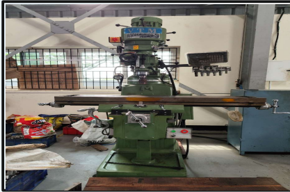
Precision Milling Machine 1270x254mm
