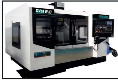
COSMOS CVM-640 (GRA PHITE) - PLAN X - Travels : 650 Y - Travels : 450 Z - Travels : 500
